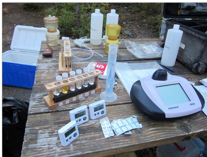
Figure 1. Set-up and equipment needed for photometer analysis in the field. The Palintest Photometer 8000 is the blue and white device at the bottom right of the picture.
