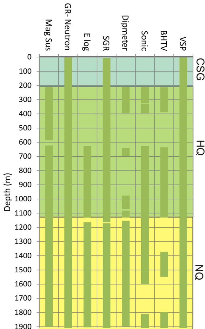
**Figure 4.** Summary of geophysical logging at Kimberley. CSG, HQ, and NQ stand for depth sections of surface casing, HQ coring, and NQ coring, respectively.
