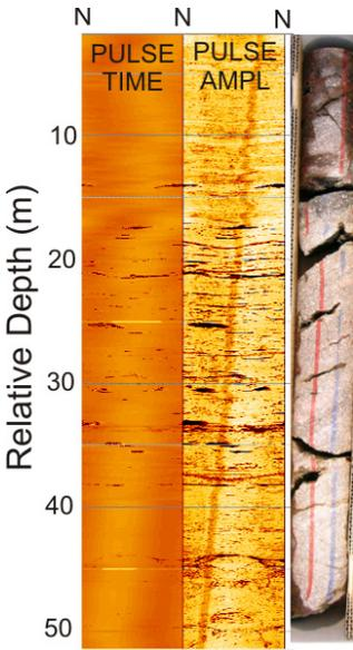
**Figure 5.** Comparison of BHTV pulse travel time and pulse amplitude images to boxed core photograph. The core length is approximately 0.6 m.
