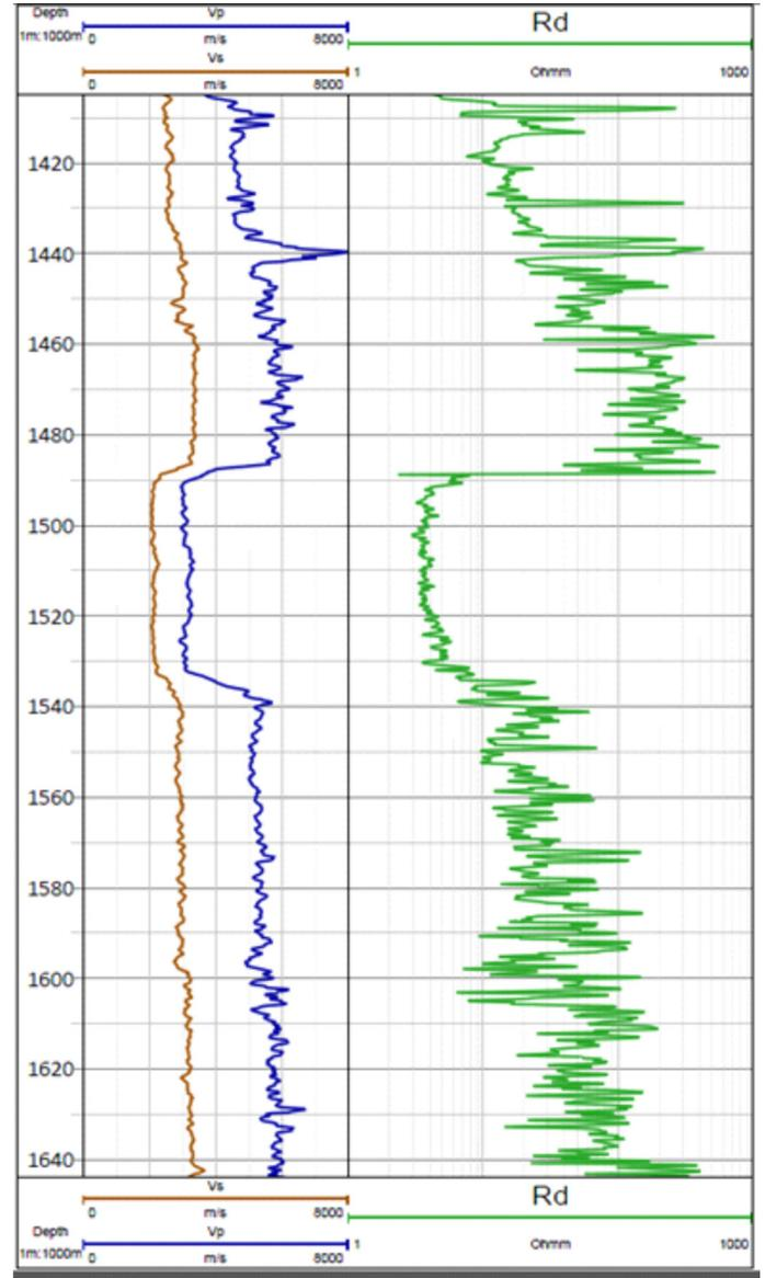
**Figure 7.** Correlations between the resistivity log (Rd) with the sonic Vp and Vs wavespeeds over a portion of the Mountain Home borehole.
