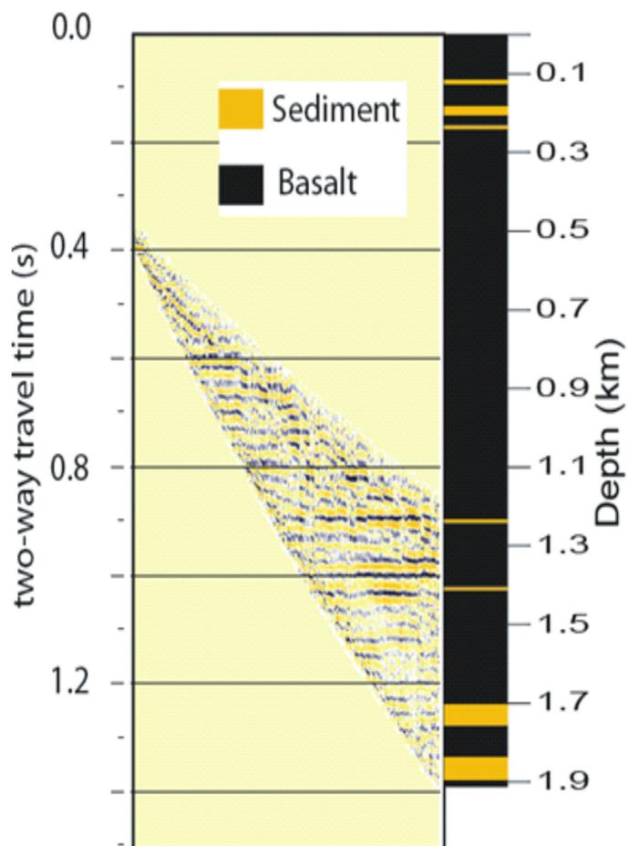
**Figure 3.** Final process 'corridor stack' obtained from the zero-offset VSP data acquired at Kimama. Strong seismic reflections are seen to be correlated with thin sediment interbeds.
