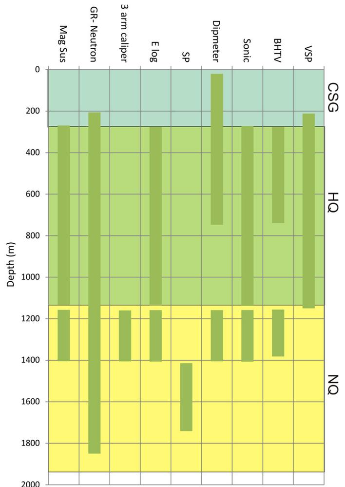
**Figure 2.** Summary of geophysical logging at Kimama. CSG, HQ, and NQ stand for depth sections of surface casing, HQ coring, and NQ coring, respectively.
