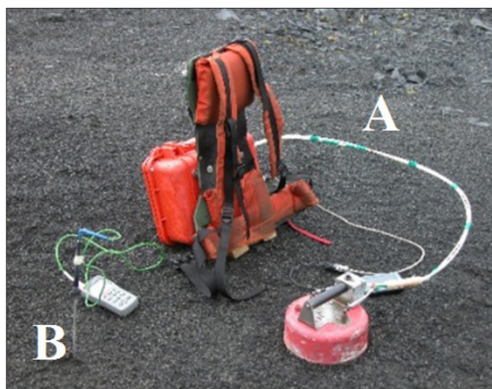
Figure 2. A) The accumulation chamber is connected via two flexible tubes (inlet/outlet) with the gas analyzer. The measurements are controlled by a wireless PDA. B) If required soil temperatures can be determined with a thermocouple.
