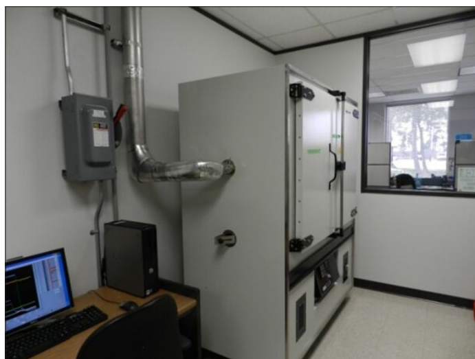
Figure 6. Images show high-temperature aging cells (left) and the 350°C (662°F) oven (right) used in the drilling fluid development program.
