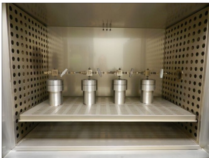
Figure 6. Images show high-temperature aging cells (left) and the 350°C (662°F) oven (right) used in the drilling fluid development program.
