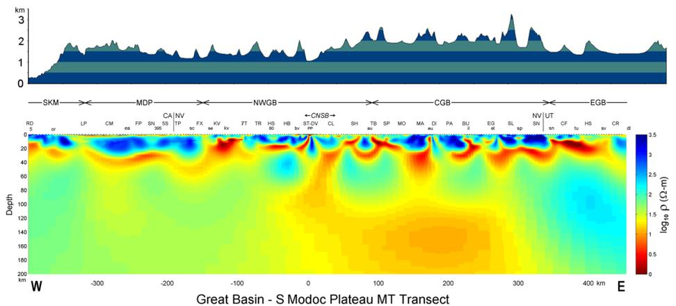
**Figure 3.** 2-D TM mode inversion section of Great Basin MT transect overlain by elevation profile. Resistivity is represented by ~22,000 inversion pixels. Geographic features defined in Figure 1 and text. SKM is Southern Klamath Mtns and MDP is Modoc Plateau.
