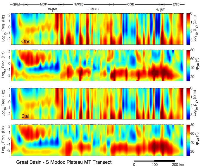
**Figure 2.** Observed transverse magnetic (TM) mode apparent resistivity and impedance phase pseudosections (upper), and model computed TM mode apparent resistivity and impedance phase pseudosections (lower) for the Great Basin-Modoc Plateau MT transect. SKM is Southern Klamath Mtns and MDP is Modoc Plateau.
