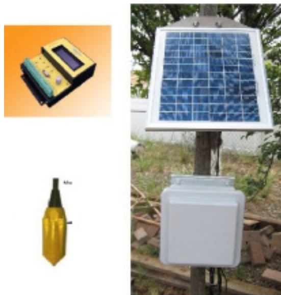
Figure 1. Data logger, top left; borehole sensor, bottom left; protective case with data logger, battery, and GPS, and solar panel, right.
