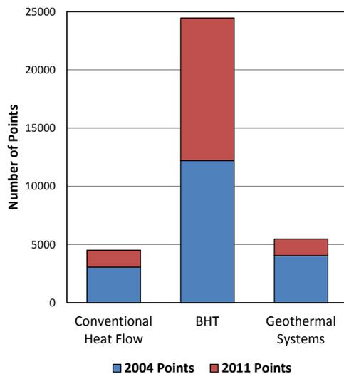
**Figure 1.** Data number and category comparison for the 2004 and 2011 heat flow maps. The geothermal category includes sites within hydrothermal anomalies that do not reflect regional conditions and were not used in the actual contouring.
