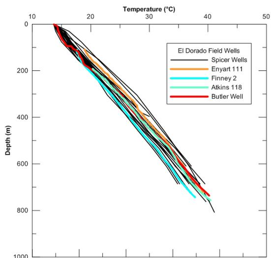
**Figure 3.** Temperature-depth data for the El Dorado Oil Field, central Kansas. The “Spicer” maximum reading thermometer data are shown as black lines and SMU equilibrium well logging data are shown as color.
