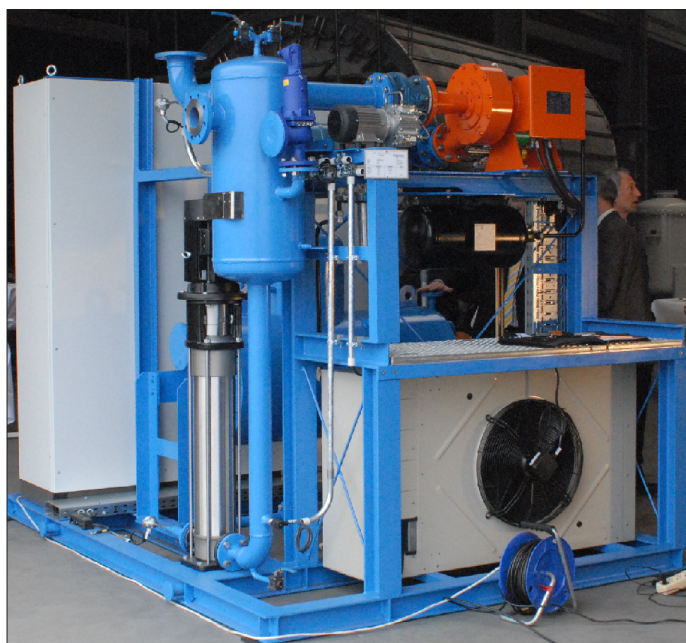
Figure 4. Small scale power plant ( 60\text{ kW}_e ) for geothermal power production in remote areas. Geothermal fluid inlet temperature: 145^{\circ}\text{C} ; Working fluid: n-Butane; Weight: 3 t, Dimensions (excl. cooling): 2.8 \times 2.3 \times 2.2\text{ m} .
