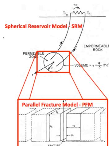
Figure 4. Spherical reservoir (SRM) and parallel fracture (PFM) models for deep EGS reservoirs.
