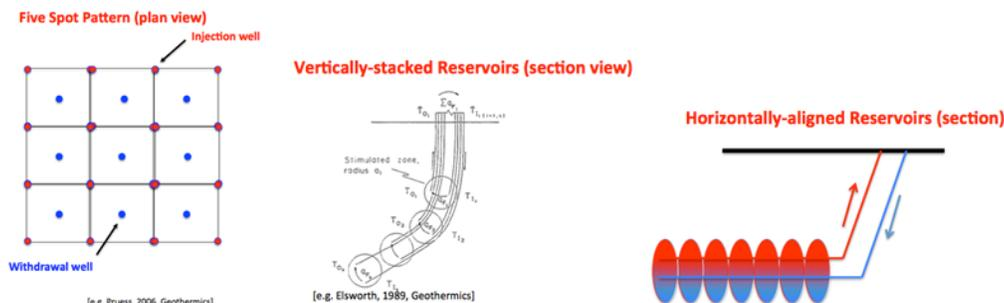
Figure 3. Five spot, and vertically and horizontally stacked reservoir configurations.
