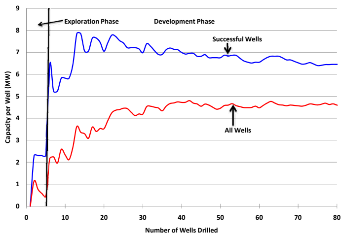
Figure 4. Average MW per Well vs. Number of Wells Drilled in Kamojang Field, Indonesia.
