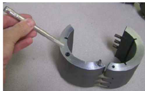
Figure 3. Maximum-registering thermometer shown with one half of the encapsulating collar assembly.
