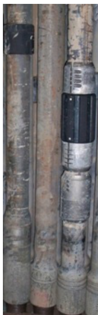
Figure 4. A conventional rotating protector installed on nearby stands of drill pipe assembly and a thermometer collar.
