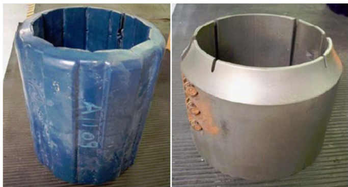
Figure 1. The existing design of a high-temperature non-rotating drill pipe protector for cased-hole. Each assembly consists of one rubber sleeve and two aluminum stop collars. The sleeve is “free floating” on the pipe between the two stop collars.
