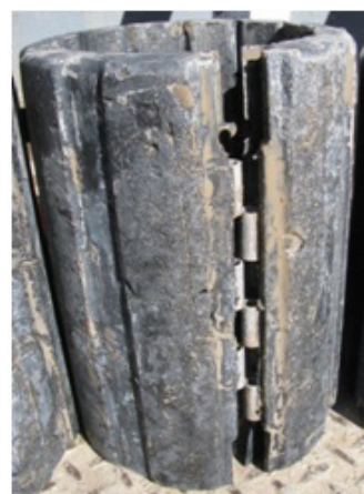
Figure 5. NRP sleeve after the initial field test, which included drilling 910 m in 130 rotating hours. Although scratched by the formation abrasion, there was no significant wear or damage to the sleeve.
