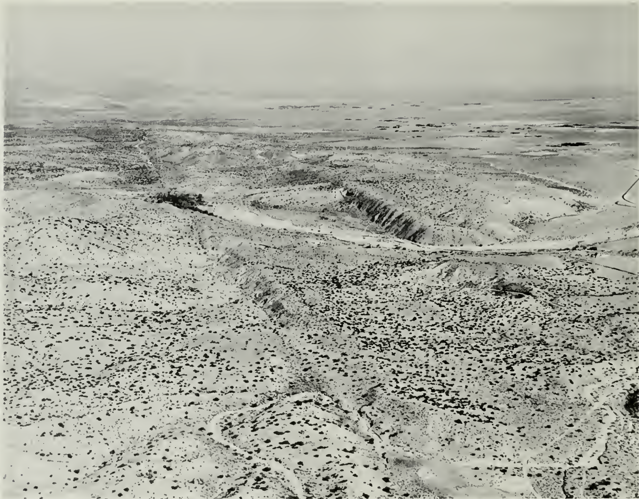
FIGURE 2. San Andreas fault zone; view northwest toward Palmdale (middle distance). Trench of San Andreas fault is at left, and scarp of Little Rock fault is at right. Exposed in the block between these parallel faults are sedimentary rocks of Pliocene and Pleistocene age; the blocks that flank the fault zone are mainly granitic rocks, with some in-faulted slices of Tertiary sedimentary rocks. Note the concentration of vegetation in Little Rock Wash where it is crossed by the San Andreas fault. Photo by J. S. Shelton and R. C. Frompton.
