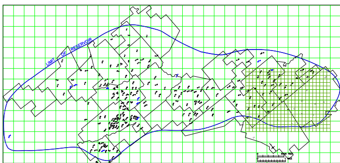
Figure 6. Grid system used in the integrated reservoir-wellbore-pipeline model.
