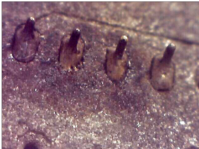
Figure 5. Photograph of solder joints in a metal-spray trace on a ceramic circuit board (after 5 temperature cycles to 250°C).
