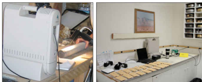
Figure 1. ASD Spectrometer in the core shack at the Blue Mountain DB2 drill site, near Winnemucca, NV. Light source illuminates the cut surface and is sensed by the lens/fiber optic "gun". On the right, the equipment in the Navy's China Lake facility with the wand attachment for measuring chips in envelopes. Chips are emptied onto a sample tray or plate for measurement.
