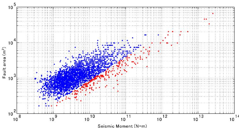
**Figure 7.** Correlation between the seismic moment and the fault area in log scale. Red dots indicate events with high stress drop (> 1.0MPa).
