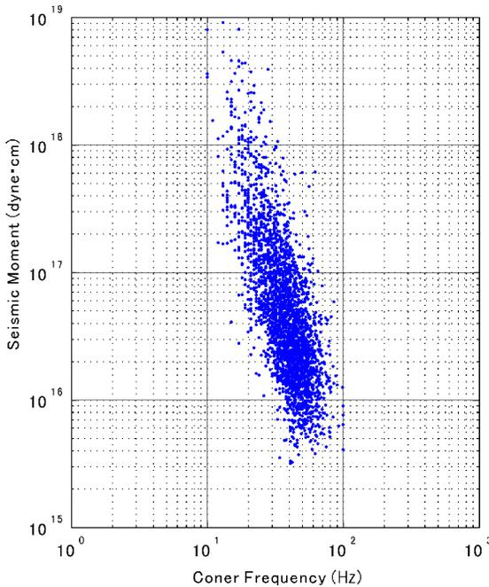
**Figure 5.** Relationship between the corner frequency and the seismic moment.
