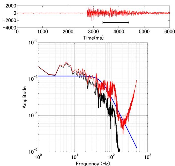
**Figure 3.** An example of waveform of microseismic event with  $M_w$  of 0.75 and observational/theoretical source spectra. Black line: the original displacement spectrum, red line: observational source spectrum, and blue line: theoretical source spectrum.
