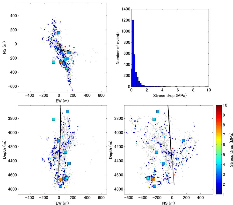
**Figure 9.** Spatial distribution of the events with high stress drop ( $>1.0\text{MPa}$ ). Color contour indicates the stress drop. Squares show the hypocenter of the large event ( $M_w > 2.0$ ).
