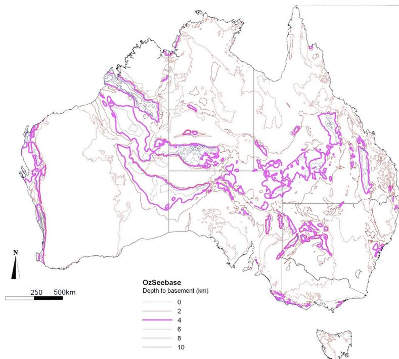
**Figure 4.** A visualization of the SEEBASE<sup>TM</sup> database. [www.frogtech.com.au/products\\_content.html](http://www.frogtech.com.au/products_content.html).
