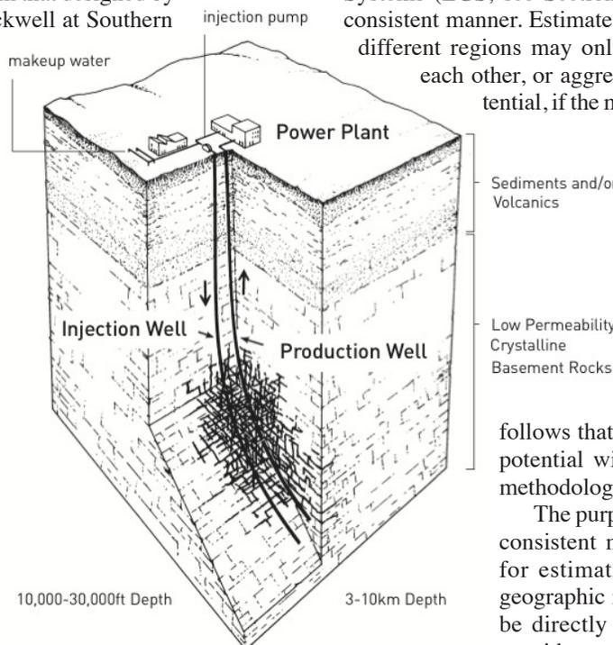
Figure 1. Conceptual EGS Power Plant Design (from MIT, 2006).
