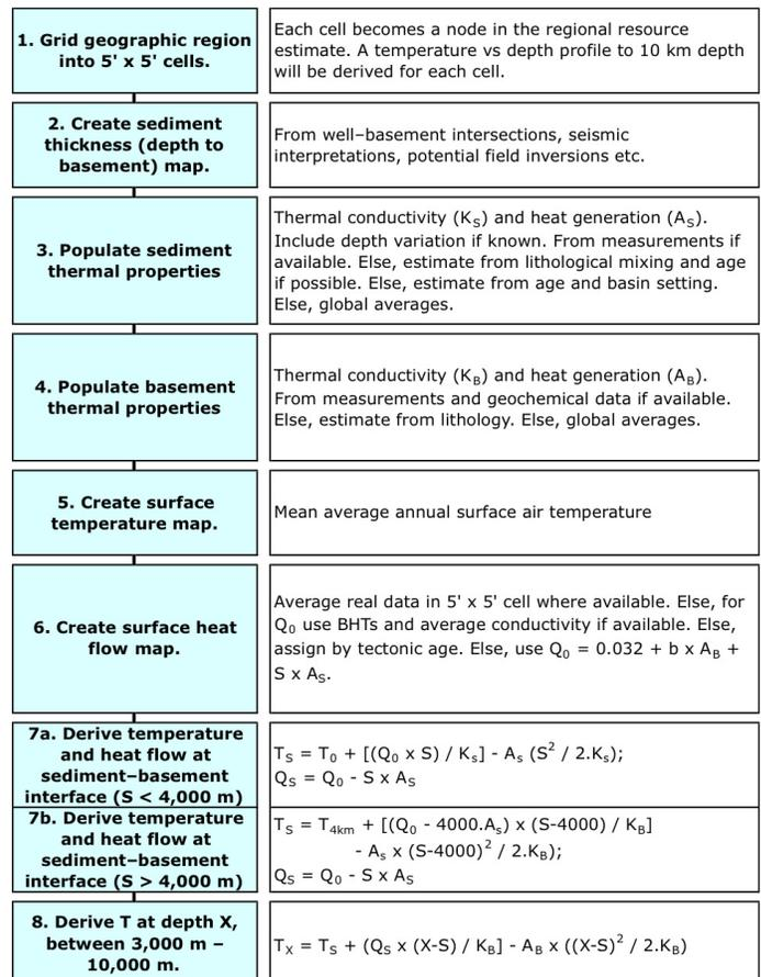
Figure 3. General process for estimating the temperature profile of the crust to 10,000 m depth.
