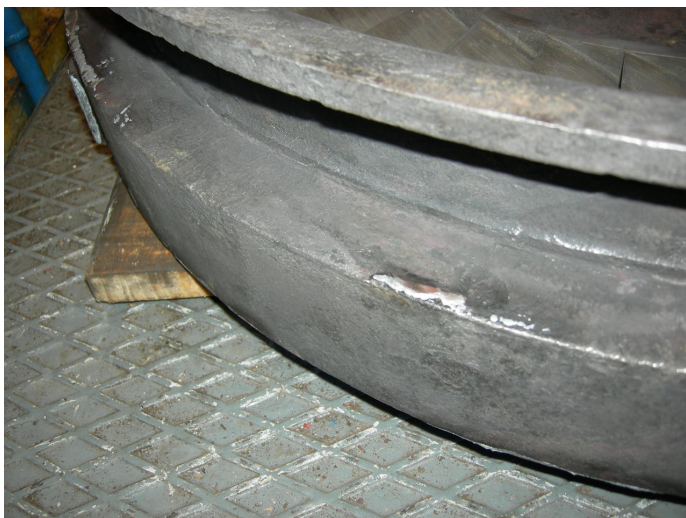
Figure 3. Diaphragm showing weld metal on the sealing face used to reposition the diaphragm axially.
