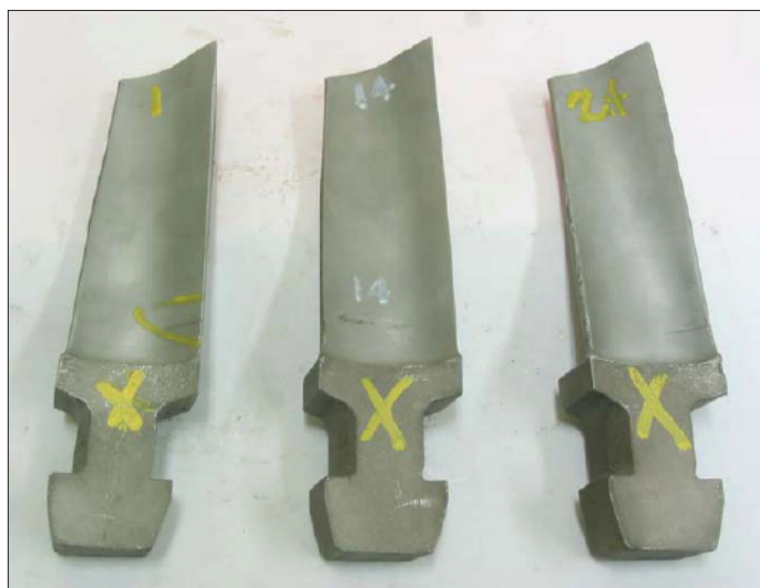
Figure 2. Cracked fifth row blades from Unit #2.
