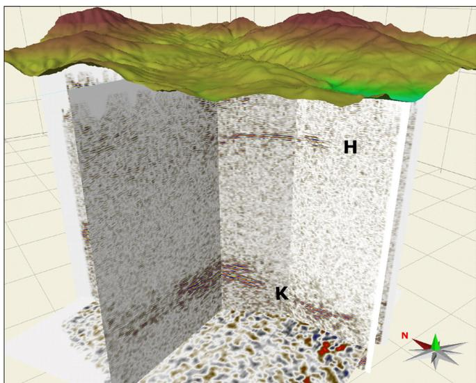
Figure 3. Seismic volume and main deep reflectors H and K.
