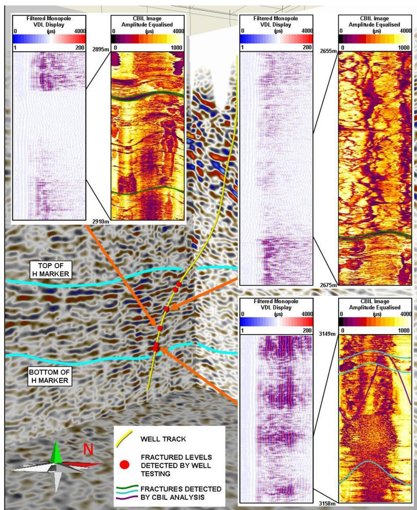
**Figure 8.** Correlation between fractured levels from well testing, 3D seismic and well log data.
