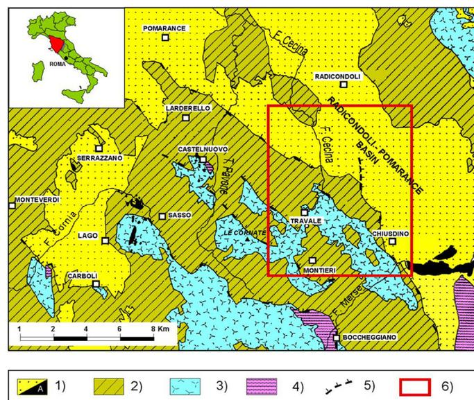
**Figure 1.** Location of the Travale test site and schematic geological map of the Larderello-Travale area. 1) Neogenic Sediments (A=Hydrothermal deposits); 2) Ligurian Flysch Unit; 3) Tuscan Nappe; 4) Metamorphic Basement; 5) Normal fault; 6) Area of the Travale test site.
