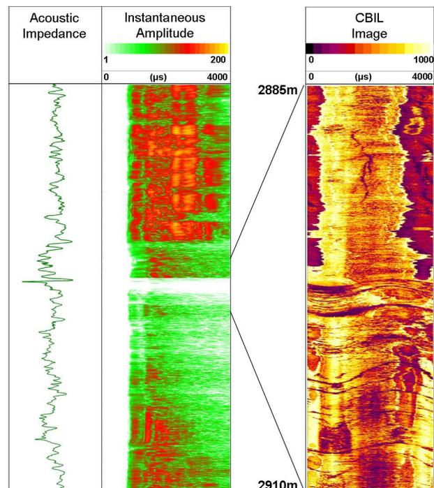
Figure 4. Fractured level evidenced by CBIL and characterized by strong absorption of acoustic energy and AI decrease.
