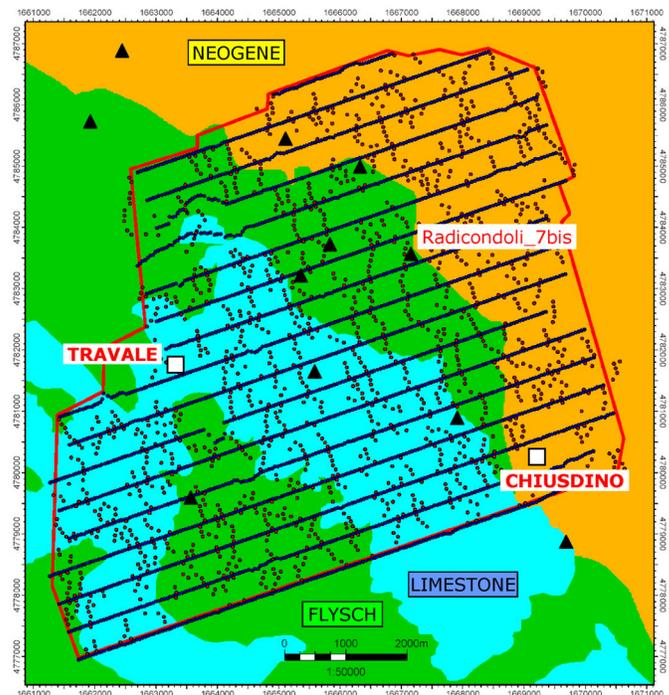
**Figure 2.** Actual acquisition layout, surface geology and main deep wells occurring in the area interested by the 3D seismic survey.
