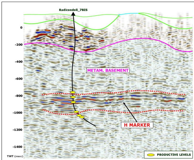
Figure 6. H marker and fractured levels identified in the Radicondoli\_7BIS deep well.
