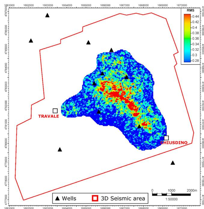
Figure 7. RMS amplitude Map of the H horizon.
