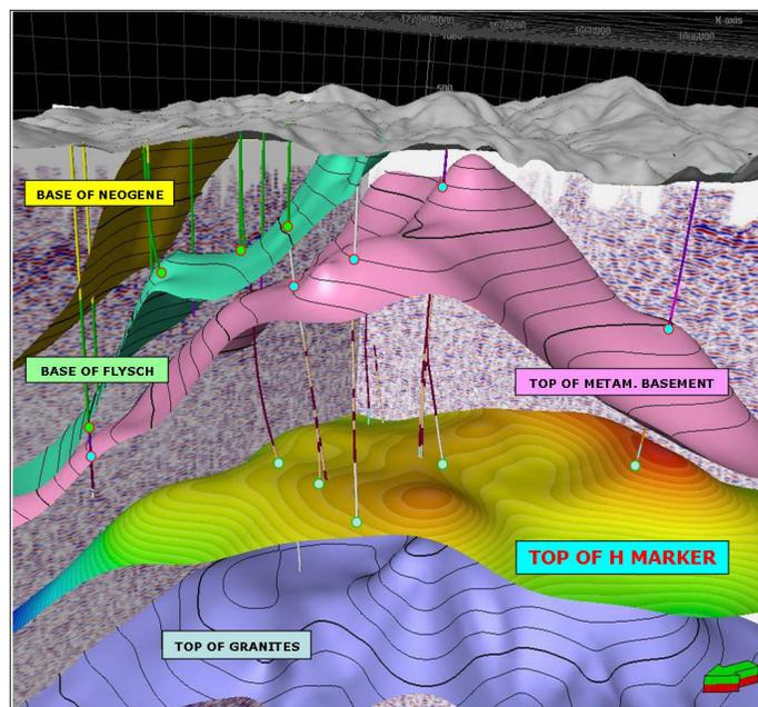
Figure 5. Main geological surfaces and seismic horizon (H and K) reconstructed from 3D seismic interpretation.
