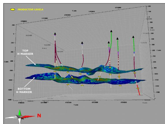
**Figure 9.** Correlation between productive levels and the seismic H horizon.
