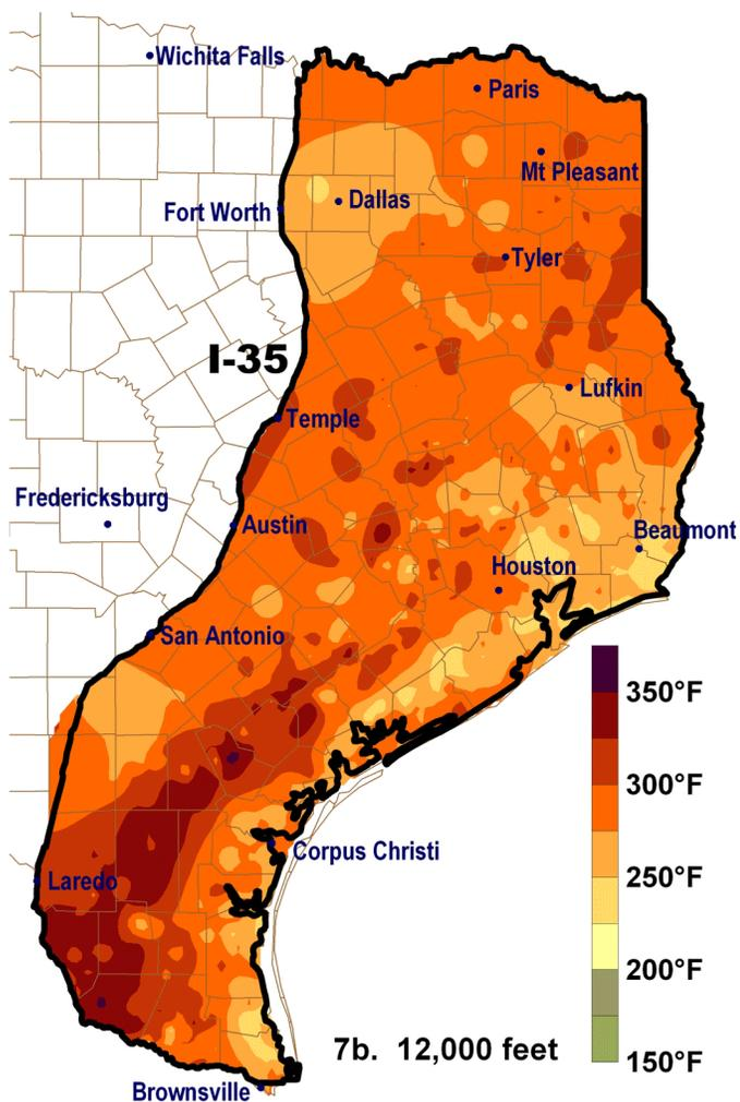
Figure 7b. Map of temperatures at 12,000 feet detailed at the county level.
