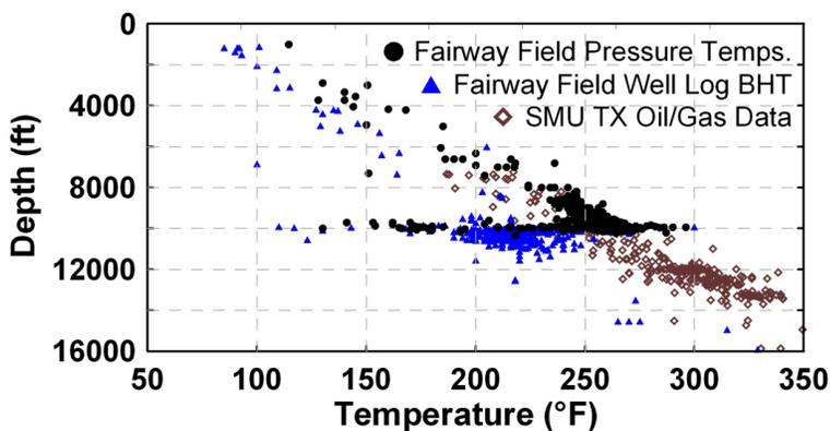
Figure 4. SMU Texas oil/gas temperature data locations within or near the Fairway Field showing the corrected values versus the averaged Fairway Field pressure data temperatures.
