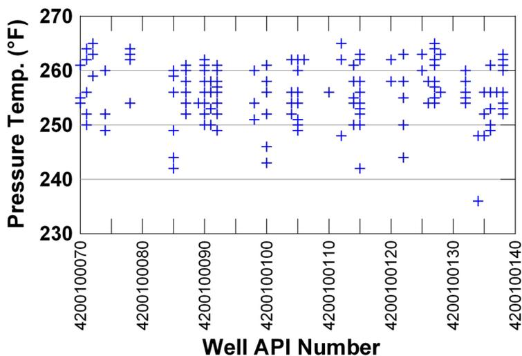
Figure 5. Fairway Field temperatures from pressure logs. Individual well sites are shown with the temperature readings over time. Each vertical line of data represents one well listed by API number along bottom axis and temperature °F on vertical axis.
