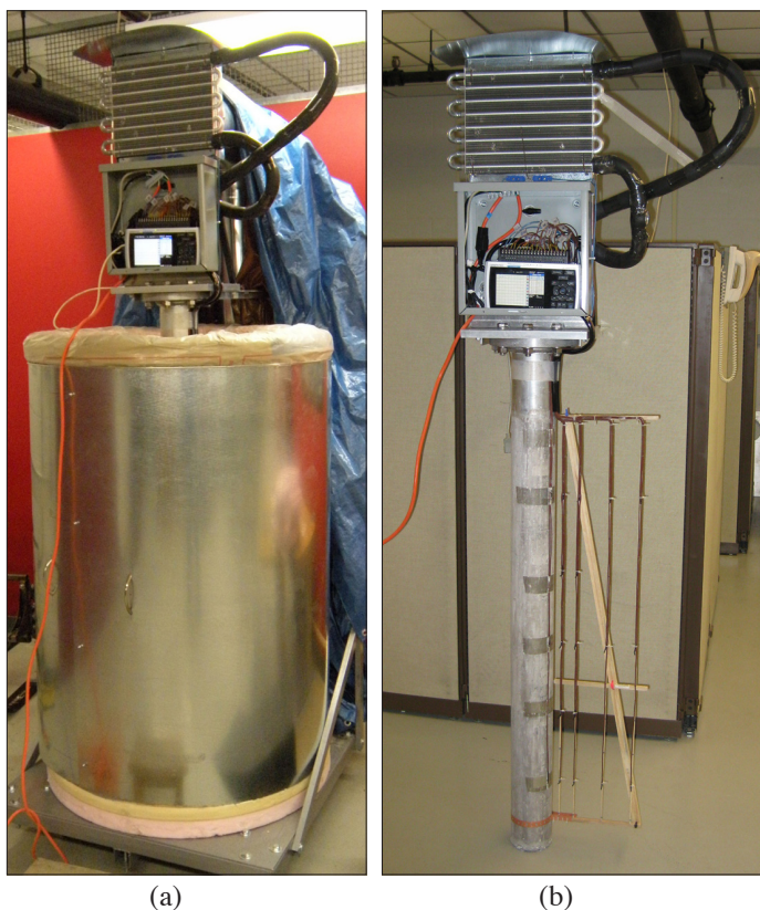
Figure 5. Smart thermosiphon in test tank (a) and removed (b) from tank to show scale and thermocouple array. The reversible thermosiphon was designed and built in the Department of Mechanical Engineering at the University of Utah.
