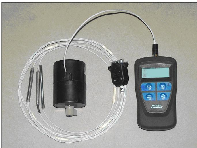
**Figure 7.** Proto type of 3 zone RTD for measuring temperatures in 2-meter probes and switch for selecting RTD at 1, 1.5, or 2 meters.
