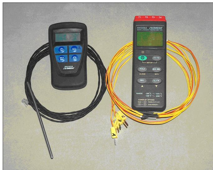
**Figure 6.** RTD and meter for measuring temperatures at 2 meter depth in probes (left), and gradient TC and 4 channel data logger for measuring temperatures at 1, 1.5, and 2 meters (right).
