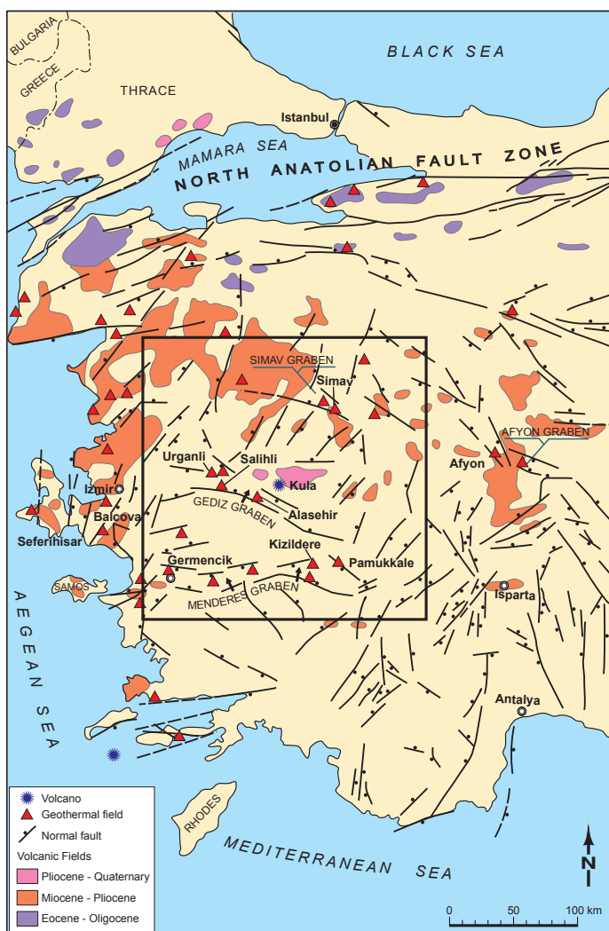
Figure 2. Generalized geologic map of western Turkey showing major fault zones and locations of geothermal systems. Black box surrounds the study area. Note the lack of Quaternary volcanism in the region. The mantle-derived basalts of the Kula volcanic field are the only Quaternary volcanics in the region.
