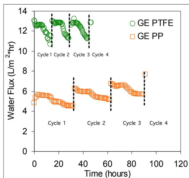
**Figure 6.** Results for DCMD performance experiments with GE PP and GE PTFE membranes. 60% recovery was achieved in each cycle. Dotted lines denote when cleaning was carried out.
