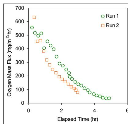
**Figure 9.** Two runs of oxygen fluxes for VMD, concentrated BD water degasification experiments with a feed temperature of 40°C.
