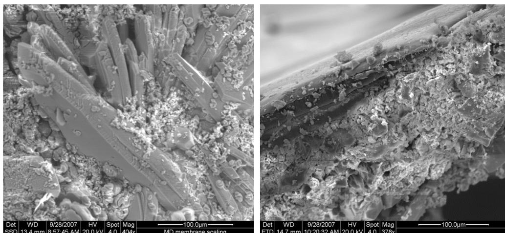
**Figure 7.** SEM images of GE PTFE membrane fouled with BD water filtered through a 0.5 µm filter. The left image is of the surface of the membrane and the right one is a cross section.
