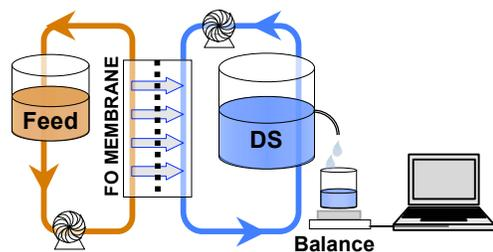
Figure 3. Bench-scale experimental apparatus for FO.
