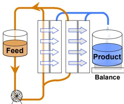
Figure 2. Bench-scale experimental apparatus for RO and NF.
