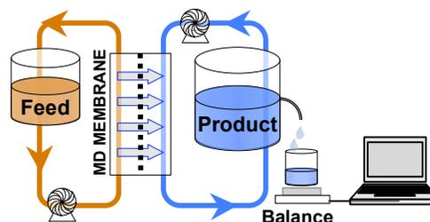
Figure 4. Bench-scale experimental apparatus for DCMD.
