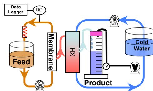
Figure 5. Bench-scale experimental apparatus for VMD.
