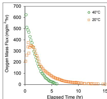
**Figure 8.** Oxygen flux for VMD pure water degasification experiments with feed temperatures of 20°C and 40°C.
