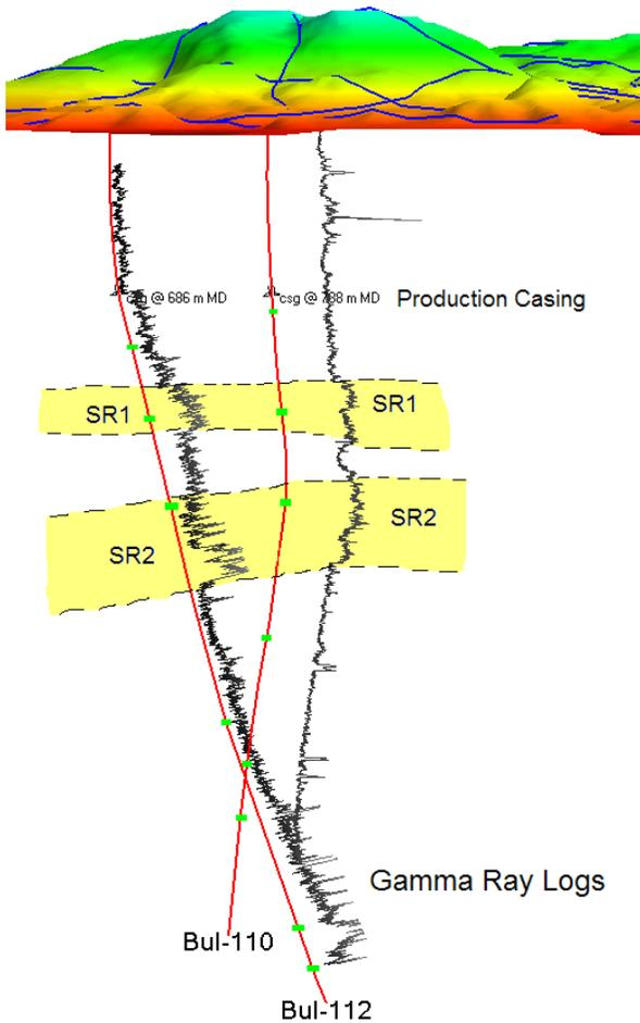
**Figure 3.** Gamma Ray log profiles in Bul-110 and -112 showing permeable zones (green markers), and the locations of SR1 and SR2.
