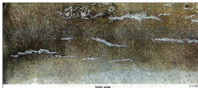
Figure 5. Stress Corrosion Cracking in CrMoV rotor.
