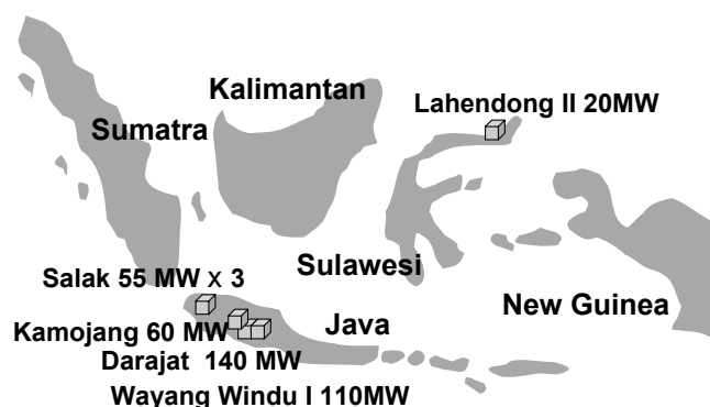
Figure 1. Geothermal power plants in Indonesia supplied by Fuji Electric Systems Co. (FES) – 3 55MW turbine-generator units in Salak, 110 MW total plant system in Wayang Windu unit 1, 55 MW and 85 MW generators in Darajat and one 60MW turbine-generator unit in Kamojang.
