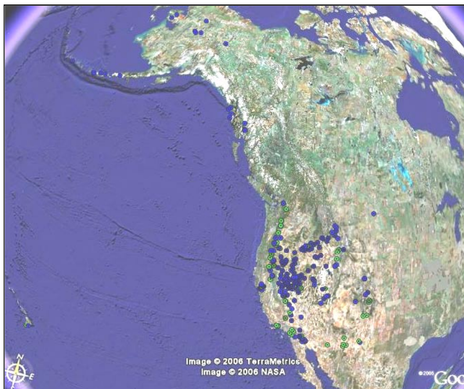
Figure 5. Hydrothermal and Convective EGS Sites Locations in the United States. Hydrothermal sites are shown in blue, convective EGS sites in green. Some of the EGS sites may be overlapped by hydrothermal sites due to the large map scale. While the site database and supply characterization covered the entire United States., only sites in the Lower 48 regions were represented for input to NEMS.
