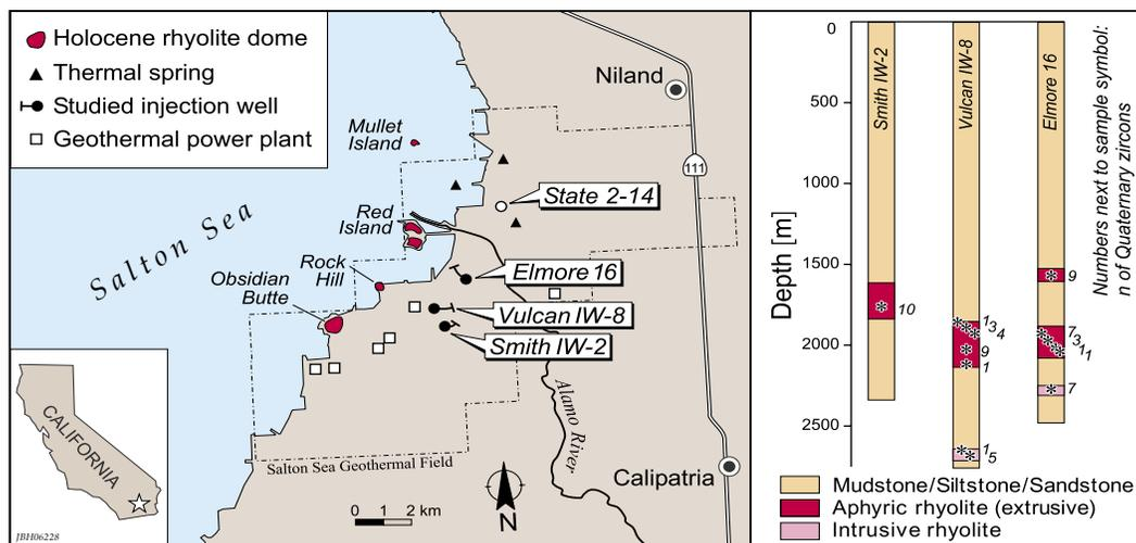
**Figure 1.** Map of surface rhyolites in the Salton Sea geothermal field (left) and simplified geothermal well logs showing subsurface rhyolite penetrations (right). Sampled intervals of  $\sim 3$  - 6 m indicated by asterisks.
