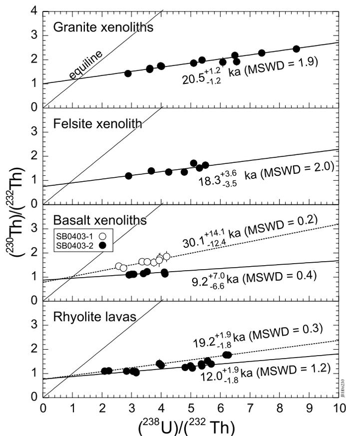
**Figure 3.**  $^{230}\text{Th}/^{232}\text{Th}$  vs.  $^{238}\text{U}/^{232}\text{Th}$  isochron plots with zircon results for surface rhyolite lavas and xenoliths from the Salton Sea geothermal field.
