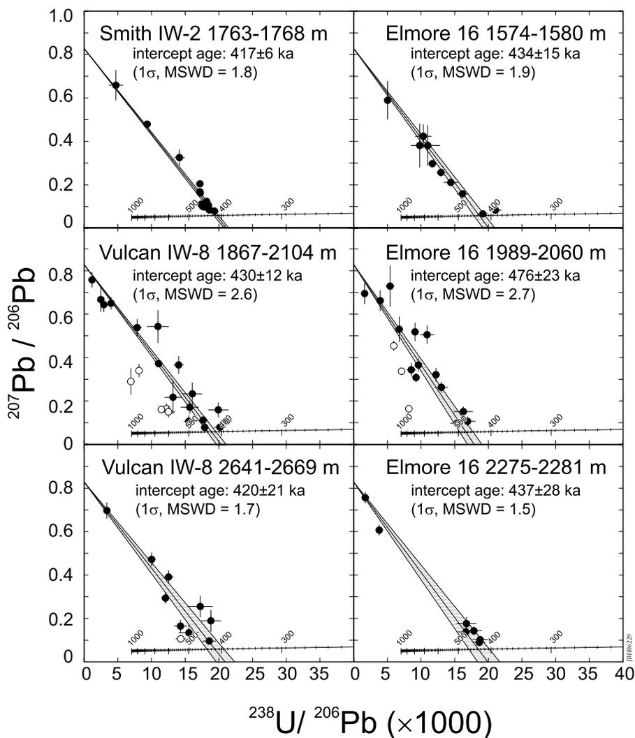
**Figure 2.**  $^{207}\text{Pb}/^{206}\text{Pb}$  vs.  $^{238}\text{U}/^{206}\text{Pb}$  (“Tera-Wasserburg”) diagram with zircon results for subsurface rhyolites from the Salton Sea geothermal field (open symbols = older grains excluded from regression).
