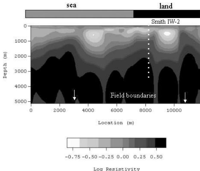
Figure 5. 2D resistivity cross-section from inverted Line 2 MT data.
