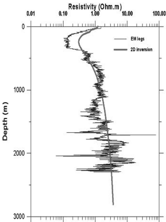
**Figure 6.** Comparison of Smith IW-2 well log and MT-based resistivity results from Line 2 of Figure 3.
