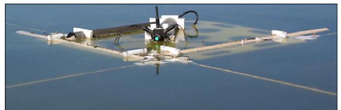
Figure 2. MMT instrumentation for shallow water (hybrid).
