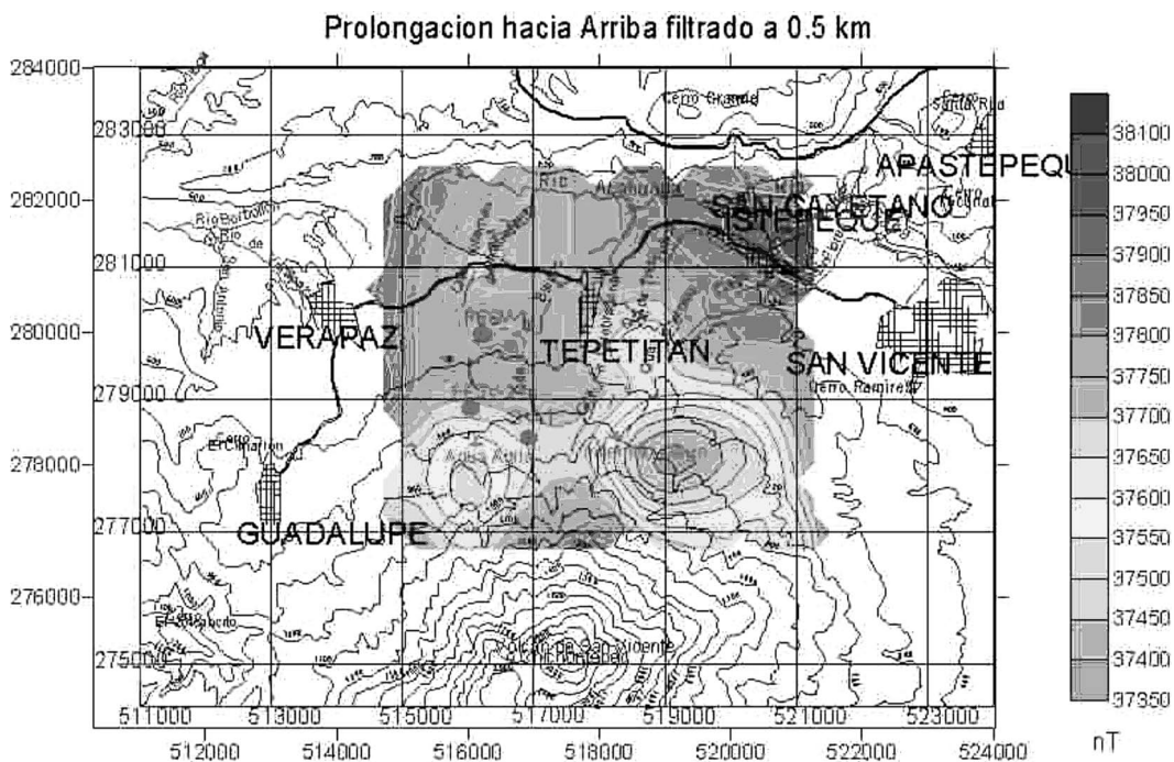
Figure 5. Upward continuation (0.5 km) magnetic anomaly map.
