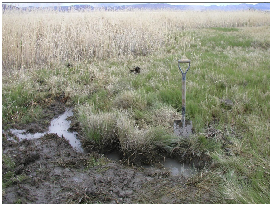
Figure 1a. A portion of the southernmost hot spring at Salt Wells. A minor amount of shovel worked helped expose a clearly defined outflow zone of hot water at 54.4^{\circ}\text{C} , which yielded a quartz (no steam loss, Fournier, 1977, 1981) geothermometer temperature of 183^{\circ}\text{C} (Table 1, sample SW-3).
