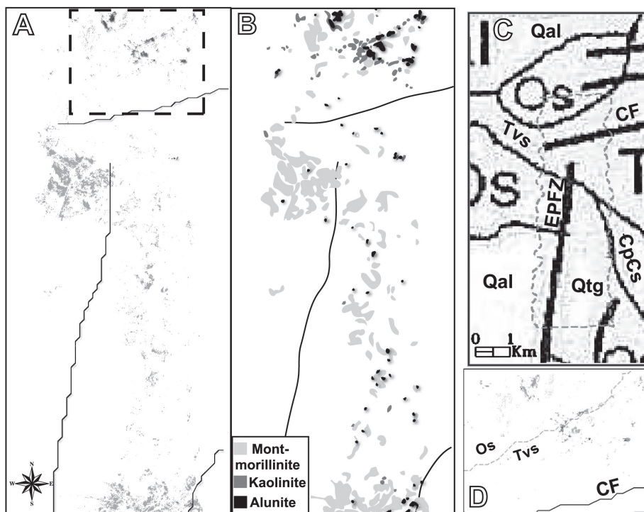
Figure 3A. Local mineral distribution map from the north-eastern portion of the hyperspectral survey. Lines represent faulting from Reheis and Sawyer, 1997. Dashed polygon shows the region highlighted in 3D. B. An attempt to clarify and simplify the mineral mapping from 3A. Minerals as defined in legend. C. Geology local to the small image subset processed in the second-tier analysis (geology from Reheis and Sawyer, 1997). Thick black lines are faults and finer lines are contact boundaries. The dashed polygon shows the actual boundary of the processed HyMap image. D. Close-up of alteration in far northeastern Fish Lake Valley highlighting coincidence of mineral formation along the Os-Tvs contact boundary (dashed line) rather than the main Coaldale Fault (solid line).
