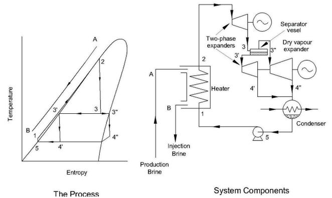
**Figure 3.** The TFC System With Divided Second Stage Expansion.
