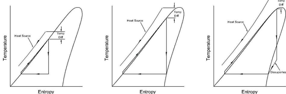
Figure 4. TFC System Expansion Changes With Increasing Resource Temperatures.
