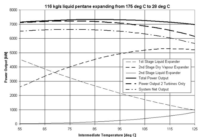
Figure 5. Power Output from Separated Flow Expander System.
