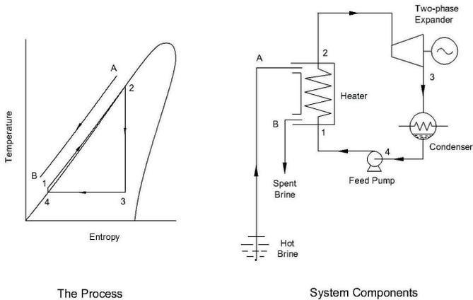
investigators, is shown in Figure 2. This has been described as a Trilateral Flash Cycle or TFC system.
