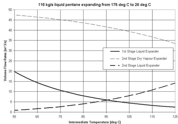
Figure 7. Exit Volume Flow rates from the Separated Flow System Expanders.
