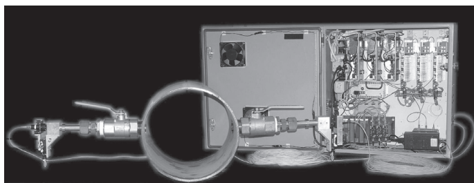
Figure 1. Monitor Instrumentation and In-situ Probes.
