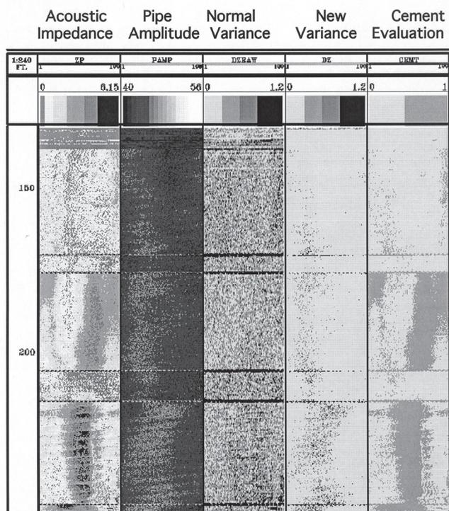
Figure 7. New technique from Halliburton for removing the effect of pipe roughness from the variance calculation. Low amplitudes are presented in the darker colors.
