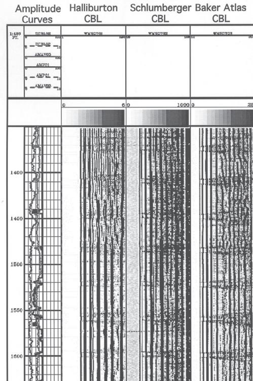
**Figure 11.** Calculated cement top from unusual means suggests the VDL or MSG variance presentation from Halliburton illustrates a change in attenuation at a depth near 1,470.
