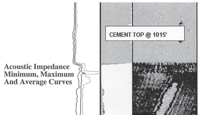
**Figure 4b.** Resulting high acoustic impedance values cause misinterpretation of cement top at annular fluid level.
