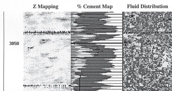
Figure 12a. Impedance Too High from Thin Annulus Interference.
