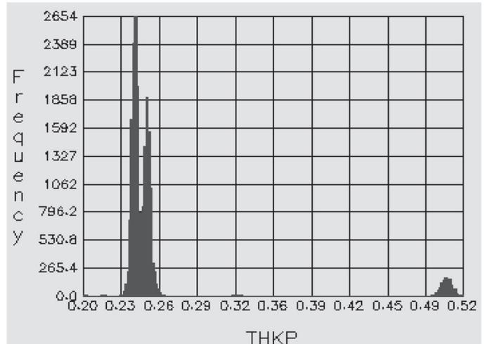
Figure 1a. Incorrect transducer frequency and location produced an inaccurate thickness measurement with a test pipe.
