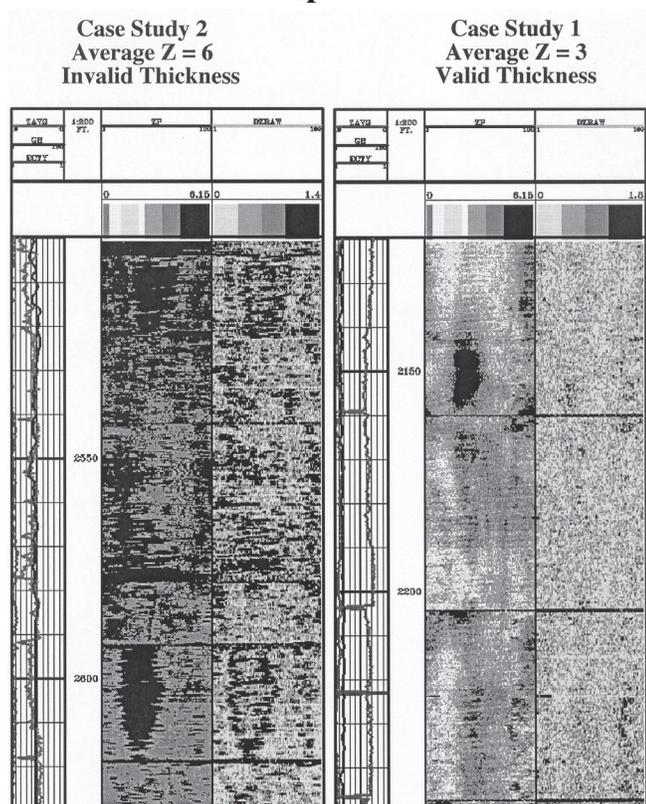
Figure 2. Acoustic impedance values unrealistically high for wellbore conditions and cement.
