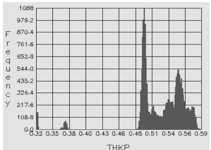
Figure 1b. Correct transducer frequency and location produced an accurate thickness measurement for the same 13 3/8 inch casing with estimated thickness of .58 inch with same test pipe.
