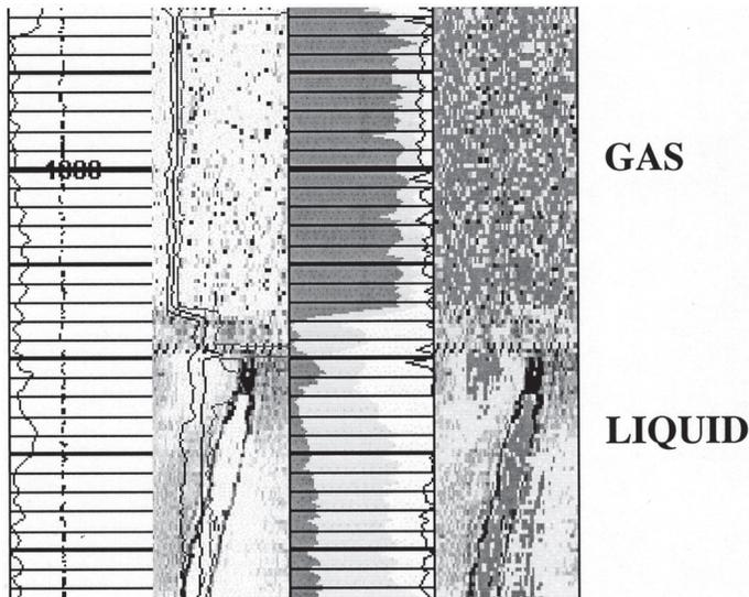
Figure 5b. Using 1.5 for drilling fluid and changing expected cement value to 2.0 from 2.6 liquid and gas are both correctly interpreted. Red or darkest shade is gas.
