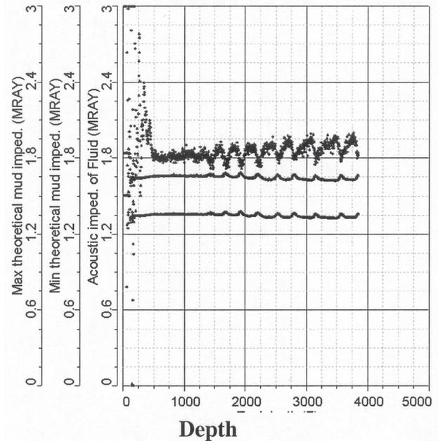
**Figure 4a.** The two lower solid lines are expected minimum and maximum values for acoustic impedance of drilling fluid. Measurement is greater than maximum value.
