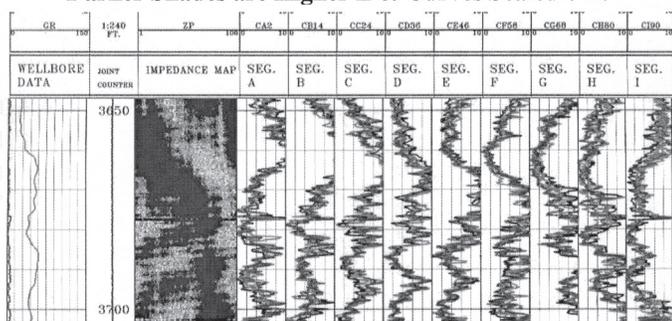
Figure 12a. Impedance Too High from Thin Annulus Interference.
