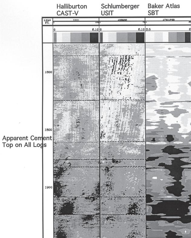
**Figure 9.** Actual cement top was higher level, but cement density was too low to be detected by normal meals between the titanium liner and steel casing.
