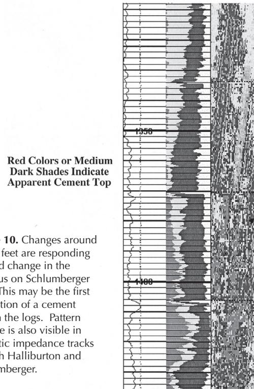
**Figure 10.** Changes around 1,370 feet are responding to fluid change in the annulus on Schlumberger log.. This may be the first indication of a cement top on the logs. Pattern change is also visible in acoustic impedance tracks in both Halliburton and Schlumberger.
