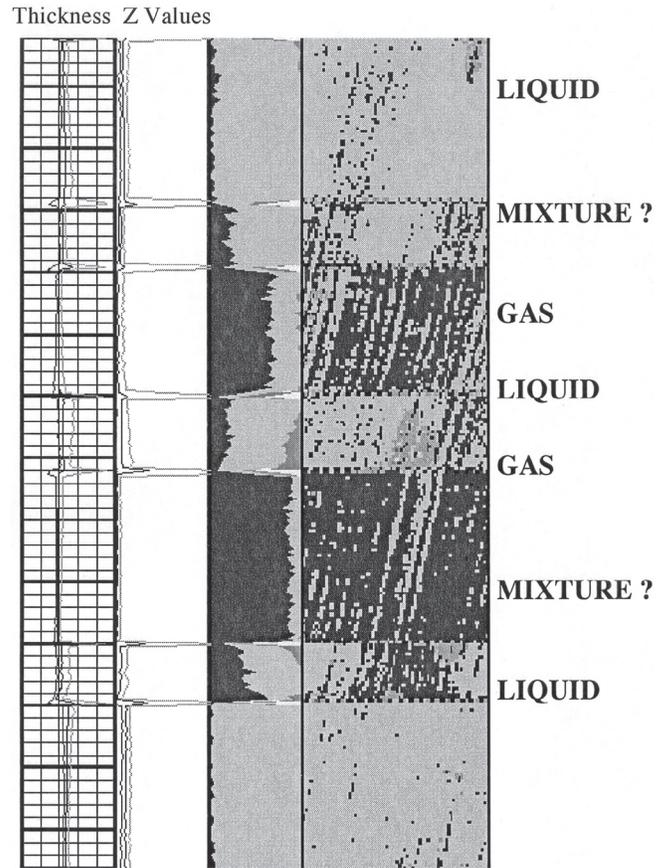
Figure 6. Interpretation 2 changes from liquid to gas based upon thickness, when annulus fluid is gas. Interpretation 3 has fewer changes by changing thickness search window.
