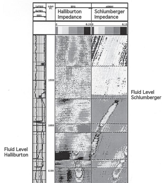
Figure 8. Both Halliburton and Schlumberger have interference patterns when liquid rather than gas is in the annular space. The water level changed between logging runs.
