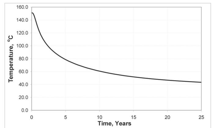
**Figure 2.** Effluent fluid temperature history for the base case in the vertical well dual perforation system.
