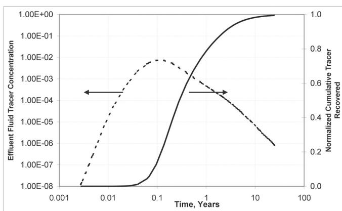
Figure 4. Effluent tracer concentration and normalized cumulative tracer recovered histories for the base case in vertical well dual perforation system.
