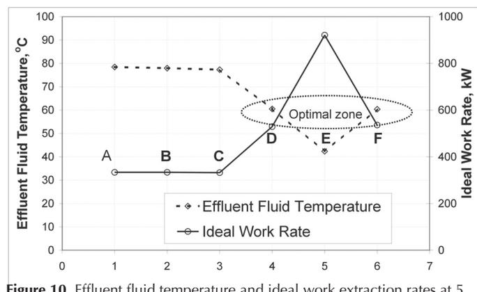
Figure 10. Effluent fluid temperature and ideal work extraction rates at 5 years as a function of parameter variation.
