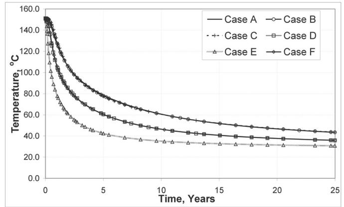
Figure 8. Effects of parameter variation on effluent fluid temperature.
