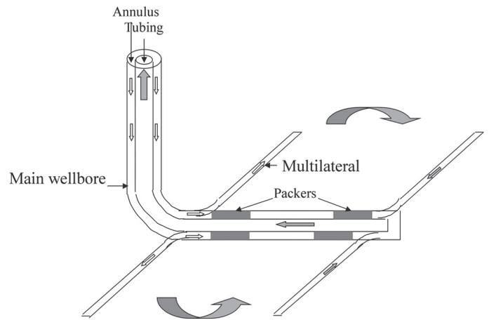
Figure 17. Schematic diagram of horizontal well multilateral doublet system.
