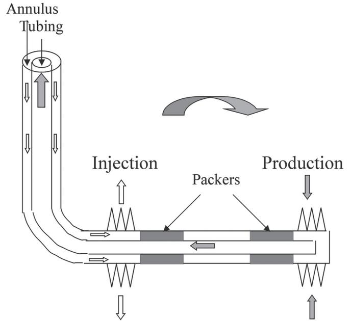
Figure 16. Schematic diagram of the horizontal well dual perforation system.
