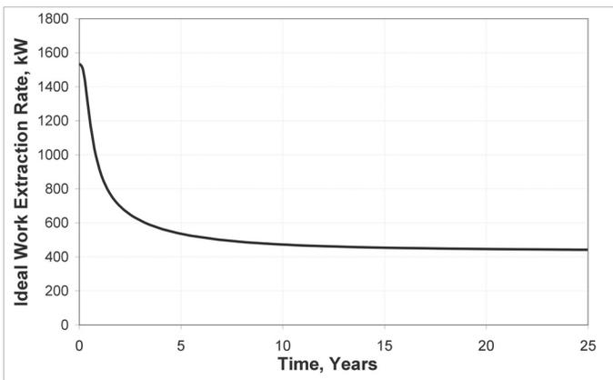
Figure 15. Effluent fluid ideal work extraction rate history for the best case in vertical well multilateral doublet system.
