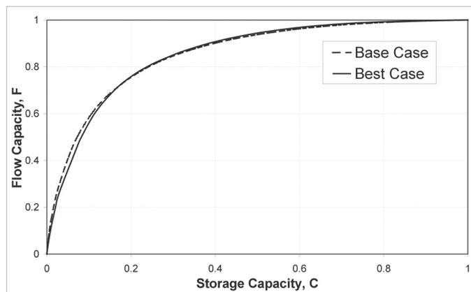
Figure 13. Flow Capacity diagram for the base case dual perforation system and the best case multilateral doublet system.
