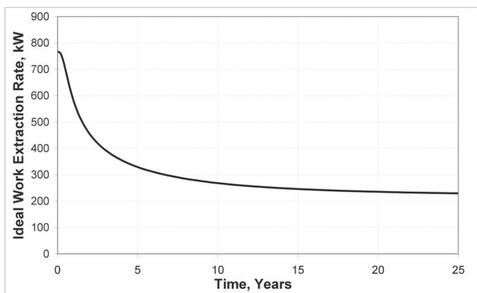
Figure 3. Ideal work extraction rate for the base case in vertical well dual perforation system.
