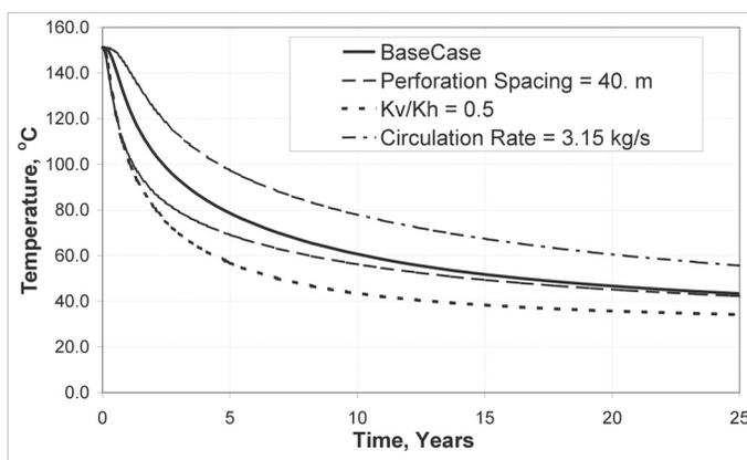
Figure 5. Effects of parameter variation on effluent fluid temperature in vertical well dual perforation system.
