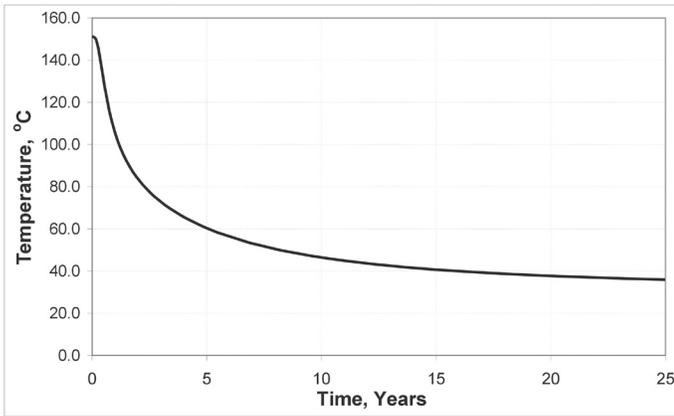
Figure 14. Effluent fluid temperature history for the best case in vertical well multilateral doublet system.
