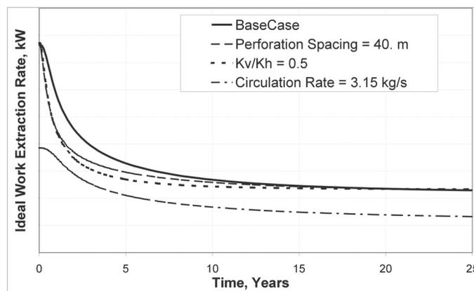
Figure 6. Effects of parameter variation on ideal work extraction rates in vertical well dual perforation system.
