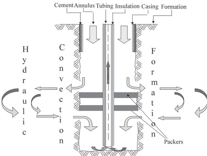
**Figure 1.** Schematic diagram of the hydraulic circulation system in vertical well dual perforation system (not to scale).
