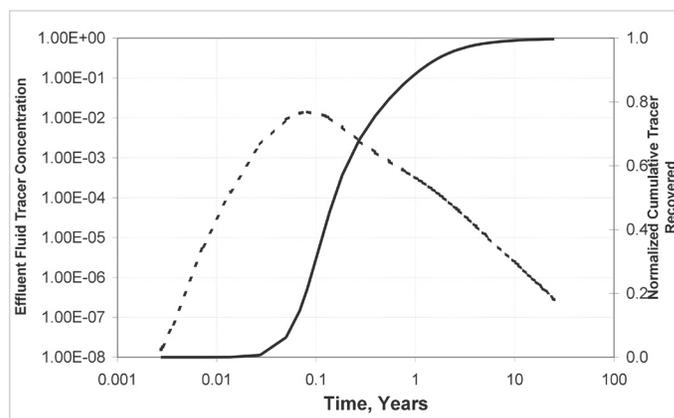
Figure 12. Effluent tracer concentration history for the best case in vertical well multilateral doublet system.
