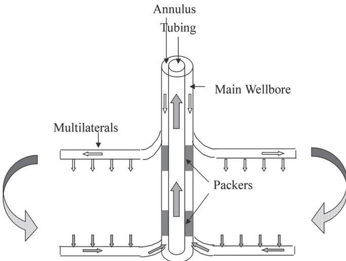
Figure 7. Schematic diagram of the vertical well multilateral doublet system. (not to scale)
