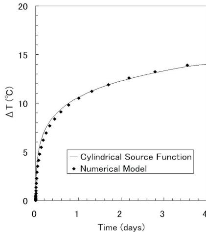
**Figure 8.** Comparison of temperatures calculated by numerical and analytical models.
