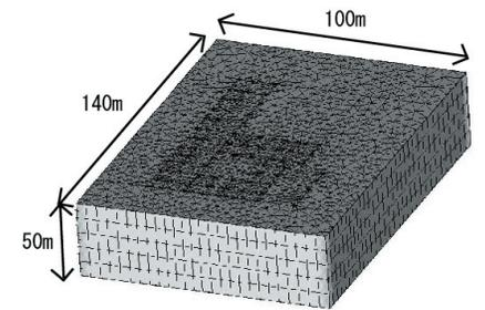
**Figure 11.** 3D view of multi-well model.
