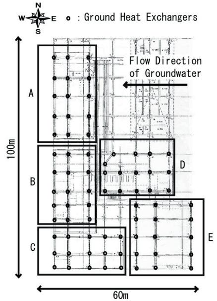
**Figure 10.** Well arrangements in multi-well model.
