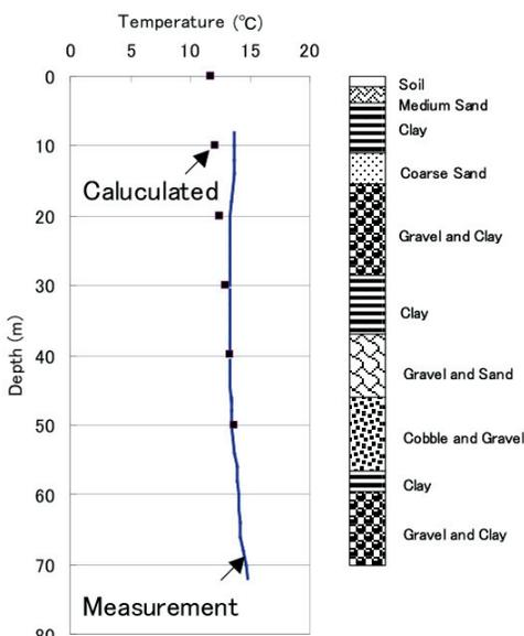
**Figure 5.** Comparison of measured and calculated well temperature profiles.
