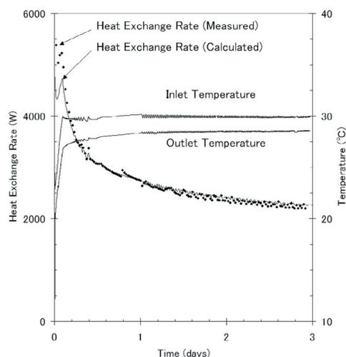
**Figure 7.** History matching result of thermal response tests.
