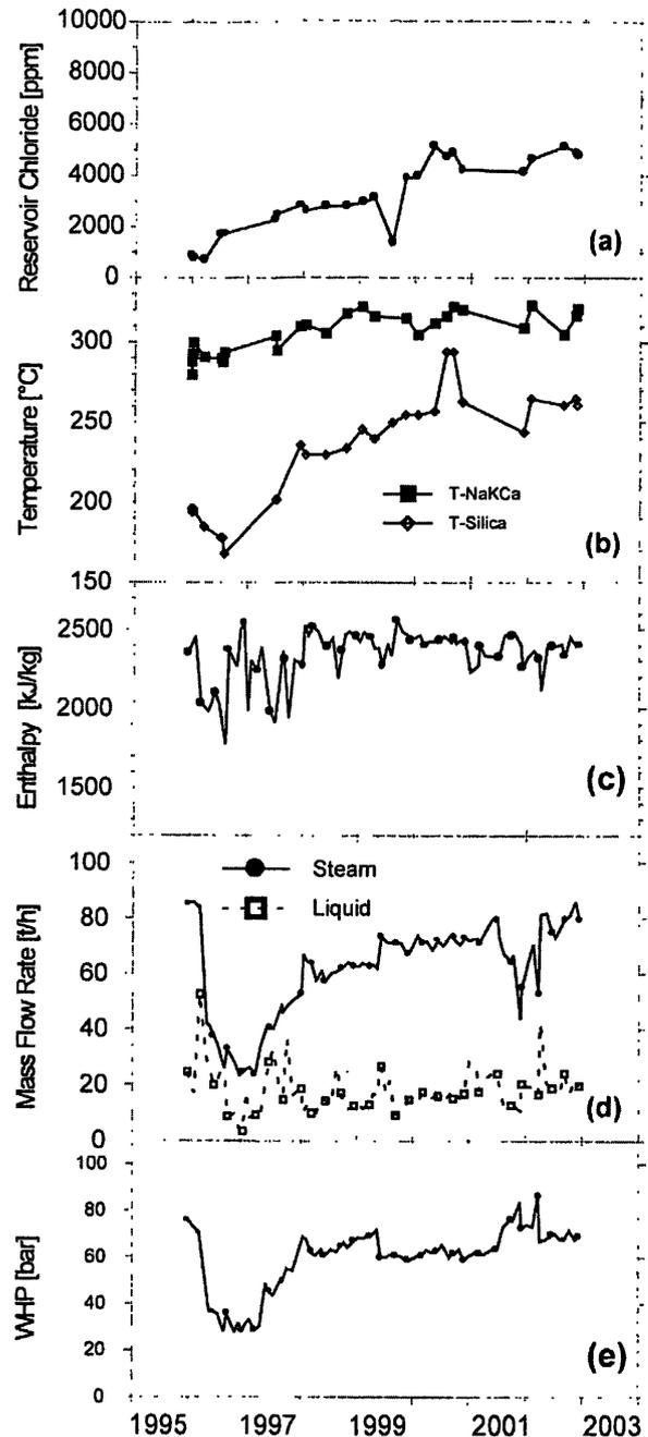
Figure 6. Well NL-1. (a) Reservoir chloride concentrations; (b) Temperatures given by the NaKCa and silica geothermometers; (c) Production enthalpy; (d) Steam and liquid flow rates at the separator; and (e) Wellhead pressure.
