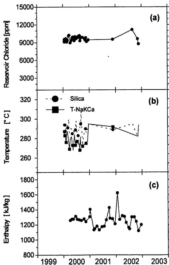
Figure 4. Well 426. (a) Reservoir chloride concentration; (b) Geothermometer temperatures; and (c) Production enthalpy.
