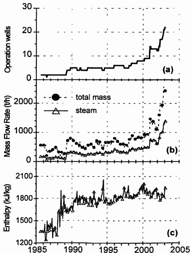
Figure 3. CP4 production history. (a) Number of production wells on line; (b) Total mass and steam flow rates; and (c) Production enthalpy.
