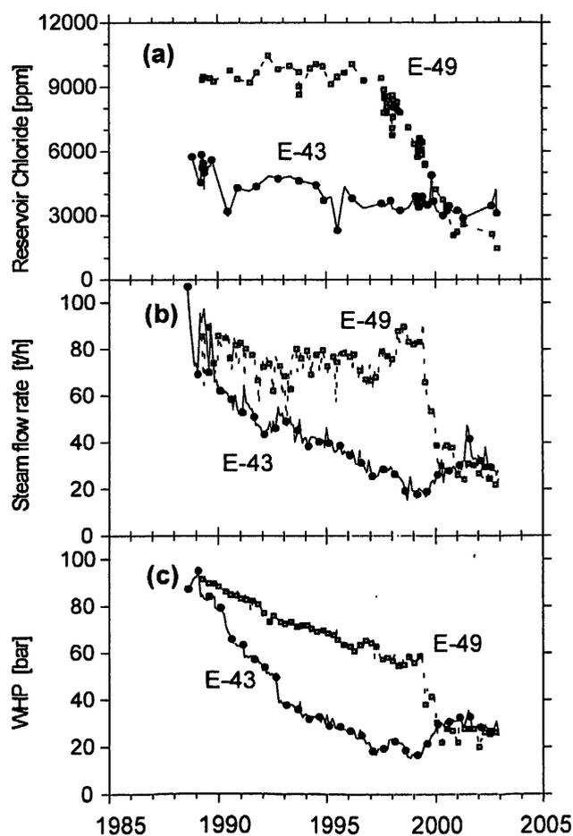
Figure 5. Wells E-43 and E-49. (a) Reservoir chloride concentrations; (b) Steam flow rates; and (c) Wellhead pressures.
