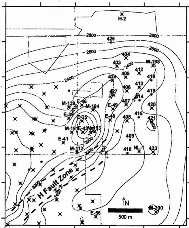
Figure 2. Depth (in meters) to the top of the silica-epidote mineral zone (SEZ) in CP4. Wells that show a continuous SEZ are indicated by an "X". In the other wells that zone seems to be discontinuous, in some cases because no cuttings wererecovered due to loss of circulation during drilling. Labeled wells are mentioned in the text.
