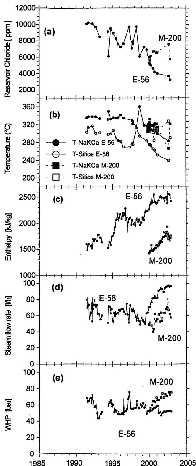
Figure 7. Wells E-56 and M-200. (a) Reservoir chloride concentrations; (b) Temperatures given by the NaKCa and Silica geothermometers; (c) Production enthalpies; (d) Steam flow rates; and (e) Wellhead pressures.
