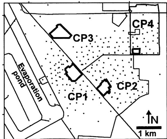
Figure 1. Location of wells (dots) and power plants (polygons with thick lines) in the four areas of the Cerro Prieto geothermal field.
