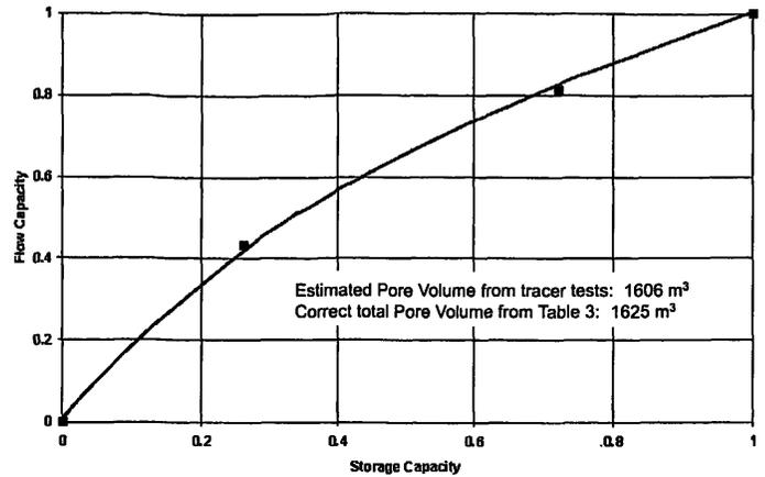
**Figure 5.** Comparison in interconnected F-C properties and those estimated from tracer data for the open boundary example.
