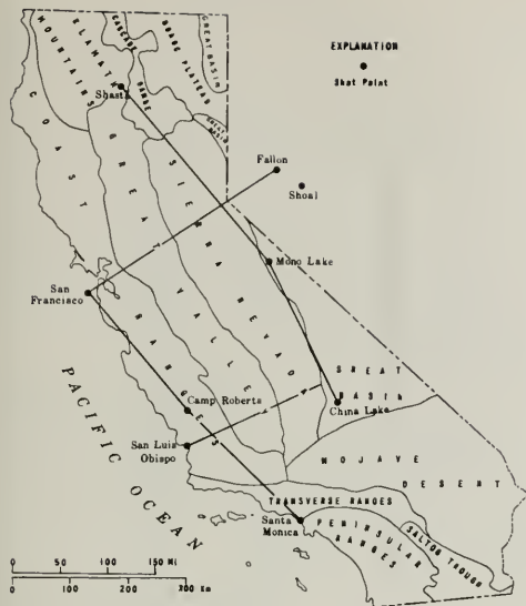
Figure 1. Map showing shot points and seismic refraction profiles made by the U.S. Geological Survey in the northern and central part of California.
