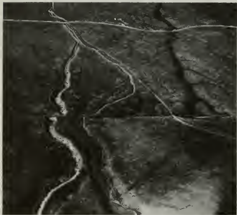
Photo 2. View southwest across San Andreas fault in Carrizo Plain, McKittrick Summit quadrangle, showing at least two, and probably three, offsets. Recent(?) right-lateral movement of nearly 100 feet is shown by abrupt bend in pair of channels in crossing the fault. Larger, and older, offset is indicated by the headless pair of channels on right, and an intermediate offset probably is indicated by less well-developed swales to left of road beyond fault.
