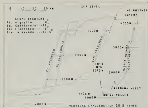
Figure 3. Comparison of three characteristic bottom profiles from the continental shelf, slope, and rise of the California continental margin with a profile of the Sierra Nevada escarpment. Modified after Uchupi and Emery (1963).
