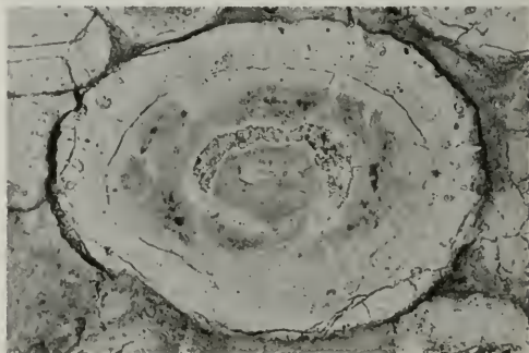
Photo 6. Core and shell of glauconite (dark) alternating with shells of collophane (light). Pellet is 1/2 mm long. Santos Shale. Chico Martinez Creek.
