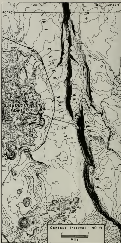
Figure 4. Topographic map of part of the Prospect Peak quadrangle, showing the Hat Creek fault scarp along the eastern edge of Hat Creek Valley. The plateau on the right of the scarp is capped with Burney Basalt. Sugarloaf Peak, on the left, is a late Pleistocene cone built largely of andesite block lava flows. The valley is floored by the Hat Creek lava flow, which only a few thousand years ago poured out of inconspicuous vents located 2 miles north of the south boundary and 1 mile east of the west boundary of the figure.
