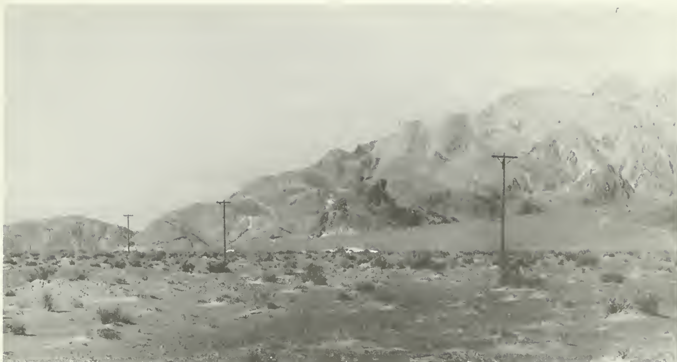
Photo 1. Lakeview Quartzite deposit: View northwest along the strike of steeply dipping Ordovician rocks at the base of the Inyo Mountains near Dolomite. The siliceous brown beds of the Pogonip Limestone are at the right edge of the dark outcrop. The Eureka Quartzite, center, is marked by the white cuts and dumps.
