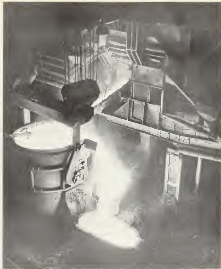
FIG. 2. Removing slag from a 90-ton ladle of molten steel at the Pittsburg, California, plant of Columbia Steel Corporation. Photo by U. S. Steel Corporation, courtesy San Francisco Chamber of Commerce.
