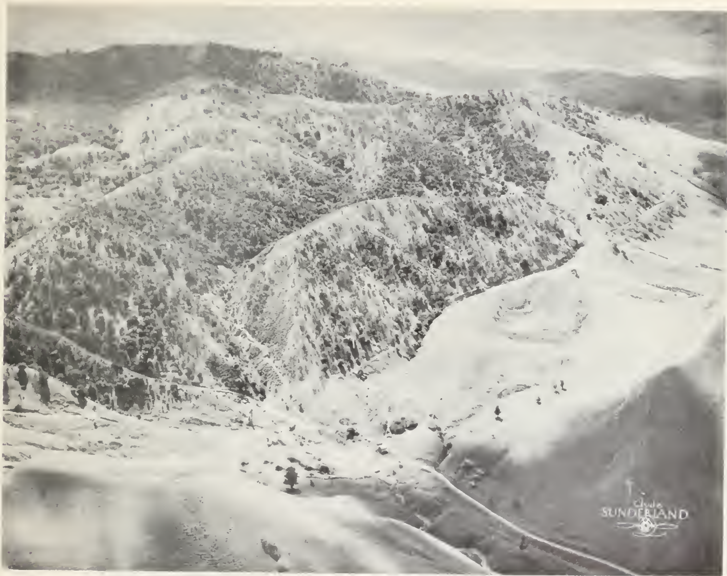
FIG. 40. Aerial view of the old coal-mining town site of Nortonville taken in 1938, camera facing south toward the base of Mount Diablo. The two mine dumps in the narrow canyon to the left of the center of the photo mark the caved entrances to two of the old workings. The low brush-covered ridge to the left of the smoke stack hides the entrance to one of the adits that is still accessible. Both the brick smoke stack and the small building in the principal mine-dump area have been demolished for the brick they contained. Since this photo was taken many thousands of tons of high-silica sand were mined from weakly cemented strata to the left of and beneath the narrow canyon floor below the two mine dumps. A partly caved stope and glory hole lead from the east side of the canyon to the floor of the next canyon east. Photo by Clyde Sunderland, Oakland.
