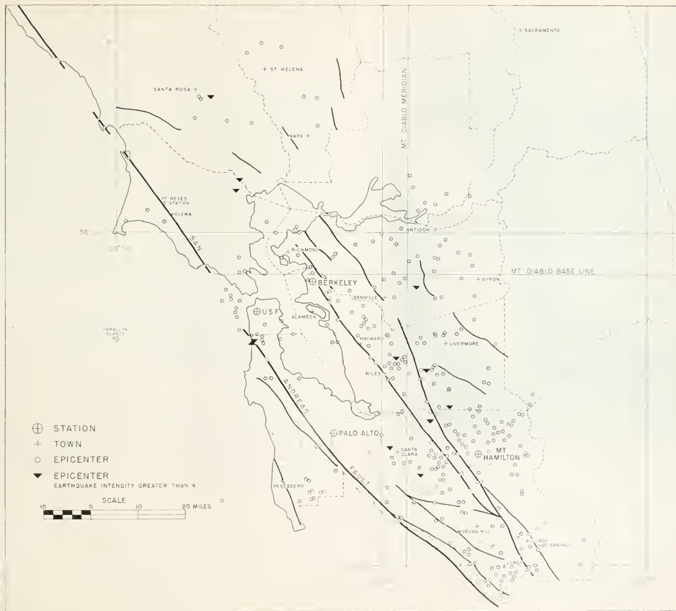
FIG. 20. Map of San Francisco Bay area showing principal active faults (heavy black lines) and the epicenters of earthquakes that occurred during the periods 1930-41 and 1947-48. The intensity of the various shocks is shown by the epicenter symbols listed in the legend to the left of the map.
