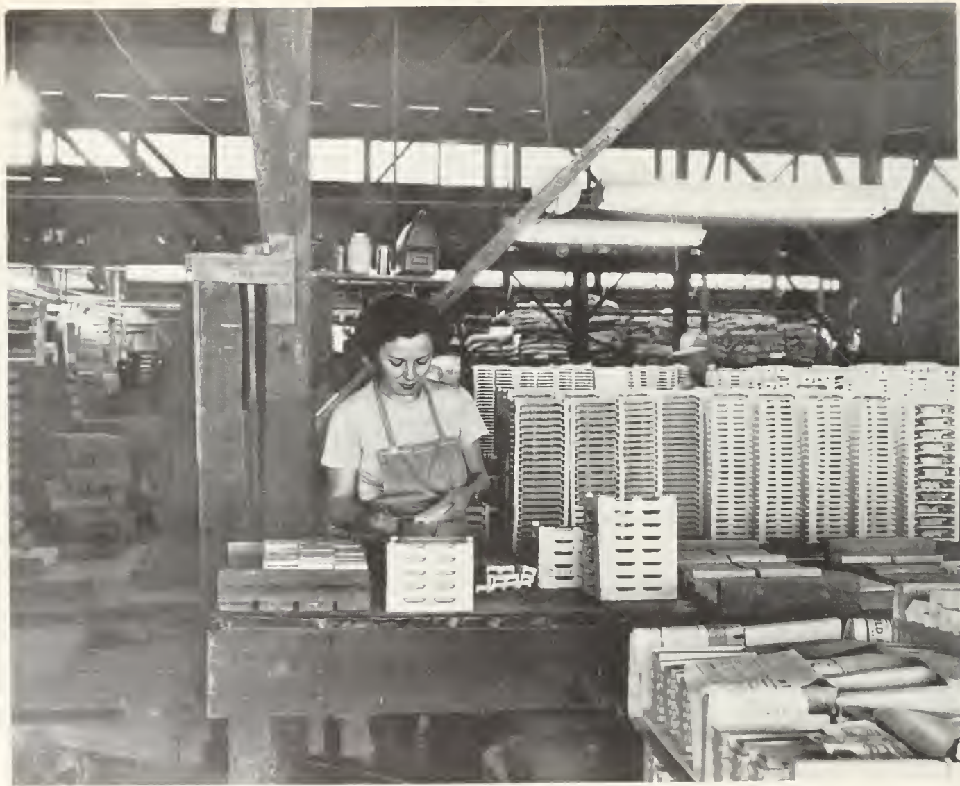
FIG. 2. Applying glaze to wall tile at California Art Tile Plant, Richmond. Photo by Mort D. Turner.
