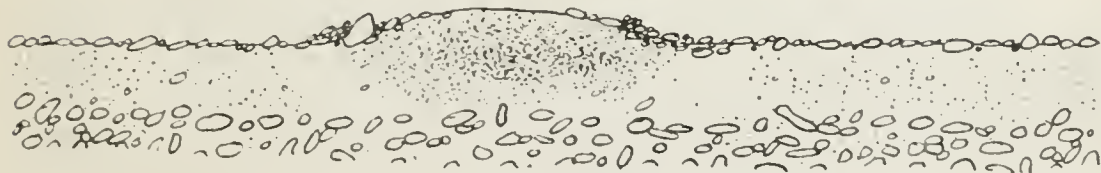
Doming has begun and pavement in center of dome has started to work outward.
