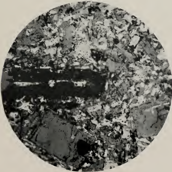
B. Anorthoclase trachyte, Tertiary (?). Large phenocrysts of anorthoclase and basaltic hornblende are set in a trachytic groundmass of anorthoclase laths, tiny biotites, amphiboles, and iron ores. Under crossed nicols, x50.
