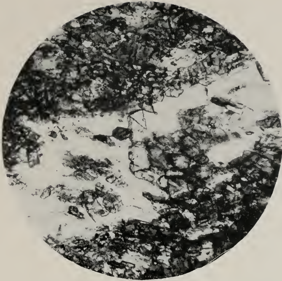
A. Actinolite-glaucophane-pumpellyite-muscovite-chlorite schist (Franciscan formation). Note large pumpellyite crystal in center; other minerals are quartz, and chlorite, actinolite, glaucophane and muscovite in the indistinguishable background. Ordinary light, x50.
