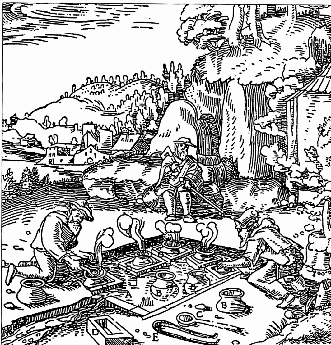
Extracting boron compounds by evaporating and concentrating boron-rich geothermal waters from natural boiling pools ( lagoni ) near Larderello, about 1540. A: natural boiling pool ( lagone ) lined with wooden boards and bricks; B: pots; C: ladles; D: wooden boxes and iron pans; E: tongs. Earthenware pots were placed in the lagoni and ladles of hot saline water were added, filling the pots half full. The water was evaporated from the pots until a thickened brine remained. Then the pots were clasped with tongs and the brine was poured into iron pans standing on four heavy legs near the borders of the lagoni . As nearly boiling hot water flowed freely around the pans, the saline brines condensed even further until the last of the water was evaporated. The mixture of boron salts was then shoveled out of the pans and the process begun anew. From De re metallica by Agricola, Italian translation by M. F. Fiorentino, H. Frobenio, and N. Episcopo. Basilea, 1563. Courtesy of ENEL SpA/Geothermal Department
